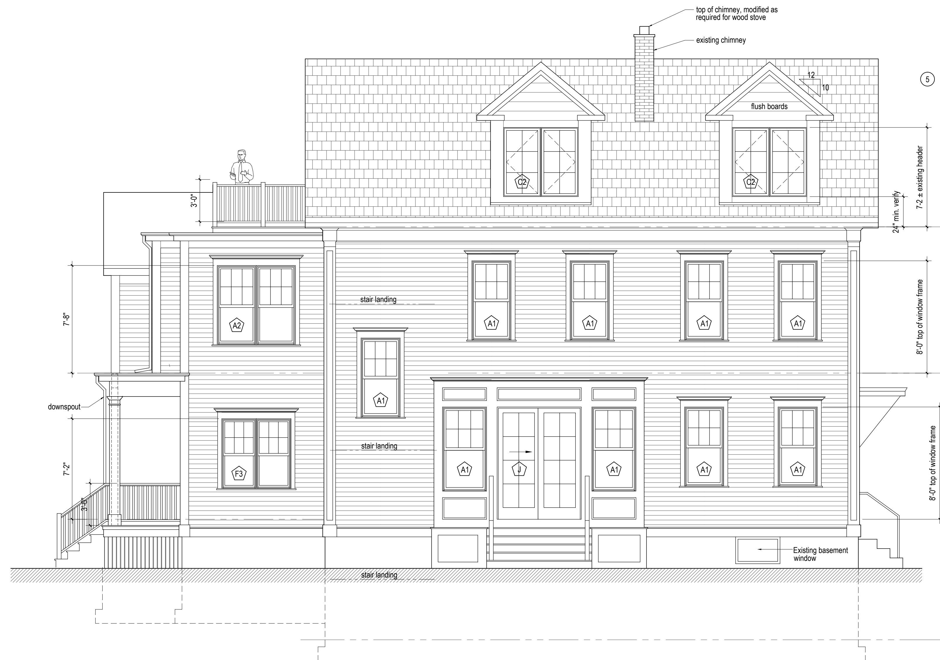
2 South (side) Exterior Elevation: 1/4"=1'-0"
