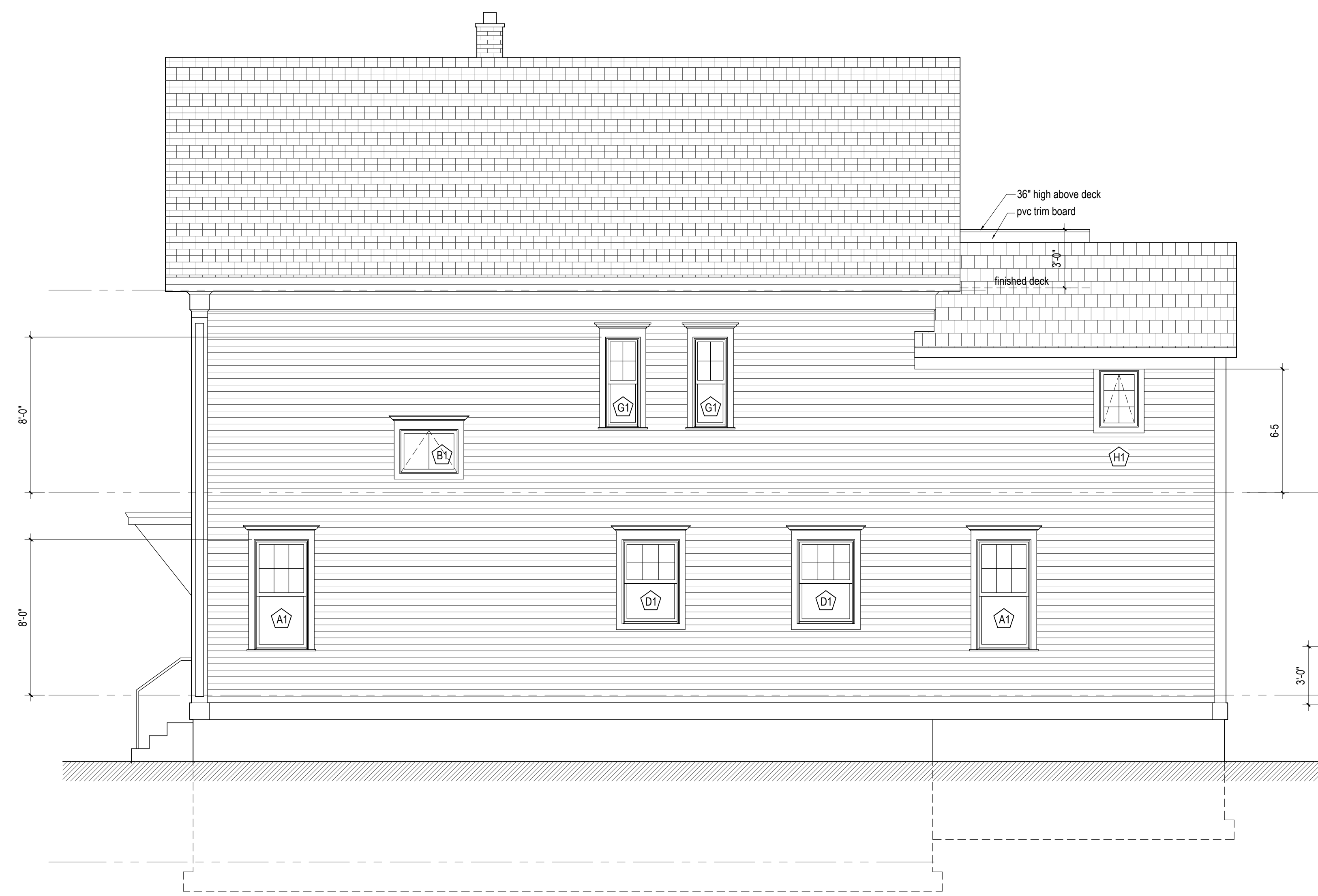
2 North (alley) Exterior Elevation : 1/4" = 1'-0"
