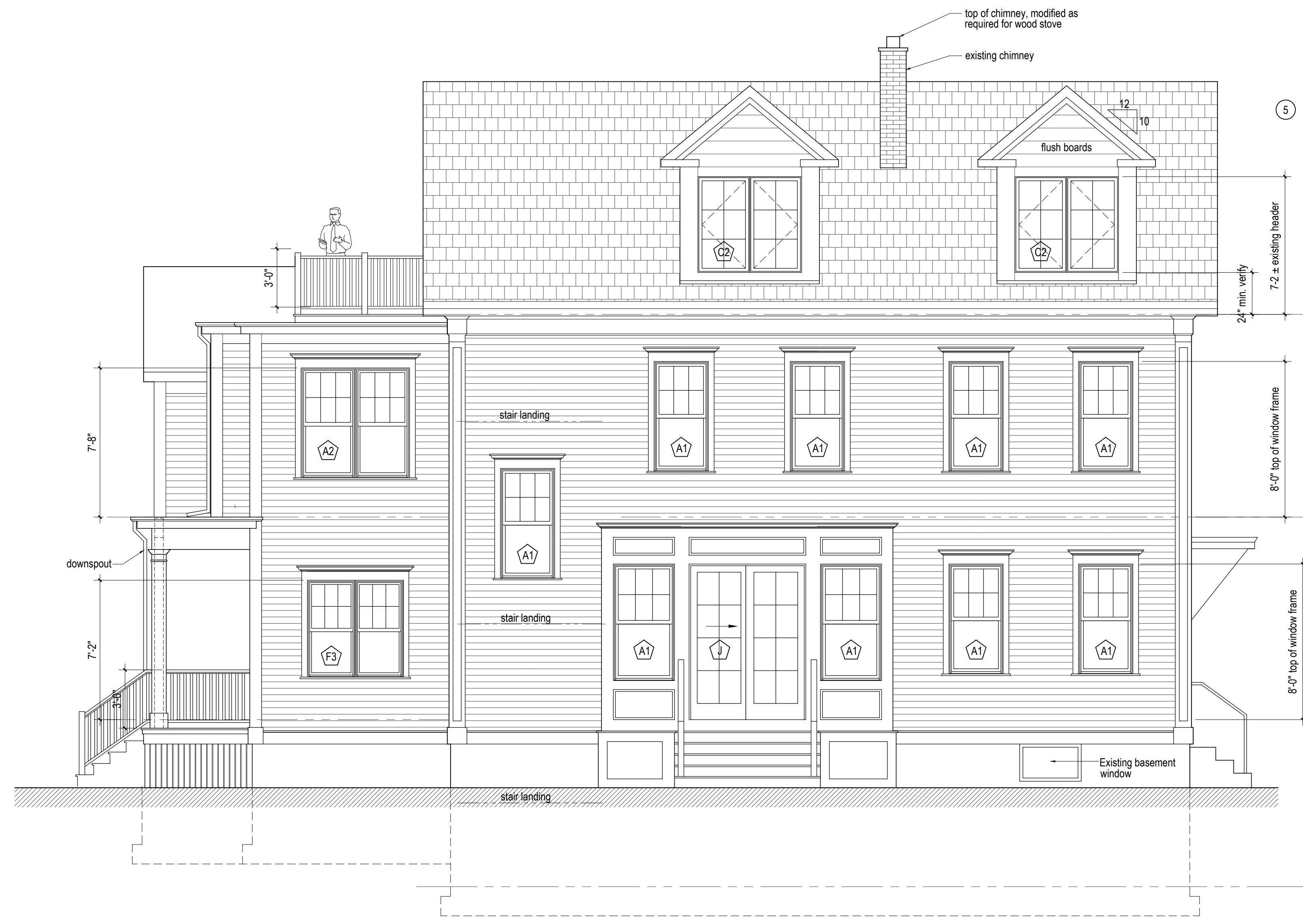
2 South (side) Exterior Elevation: 1/4"=1'-0"
