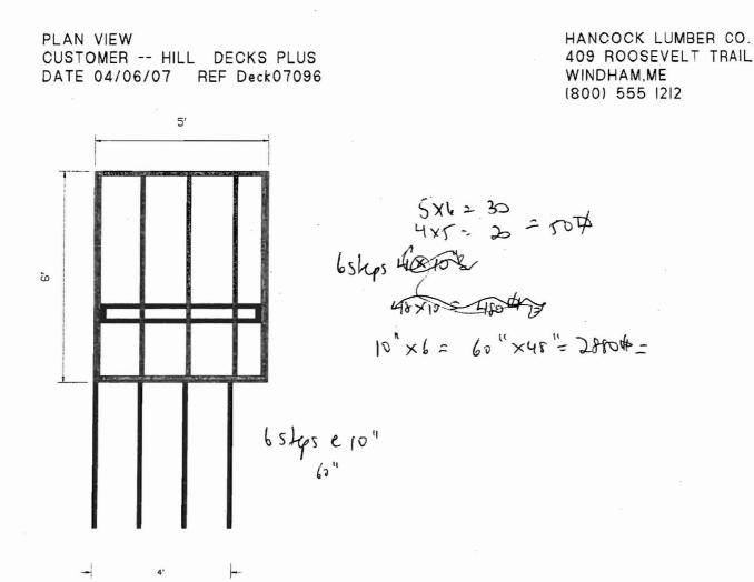
LOAD AND SUPPORT: Your deck will support a 275 PSF live load. Posts have \_\_\_ below-ground post support.
