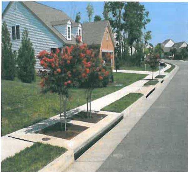
Figure 1. Filtterra ® Bioretention Stormwater Treatment System
