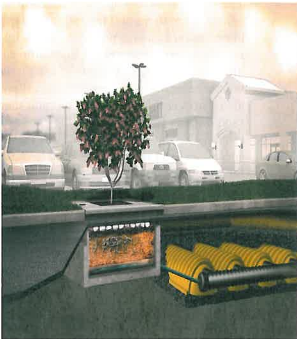
Figure 2. Typical Filterra ® Design and Installation
