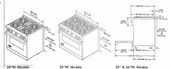
\*Add 1" to overall depth for ranges with backguards installed against a combustible wall.
