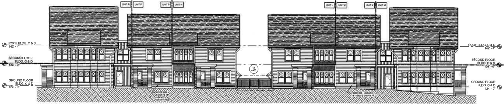
2 Condo - EXTERIOR ELEVATION SOUTH - PARK 1/8" = 1'-0"
