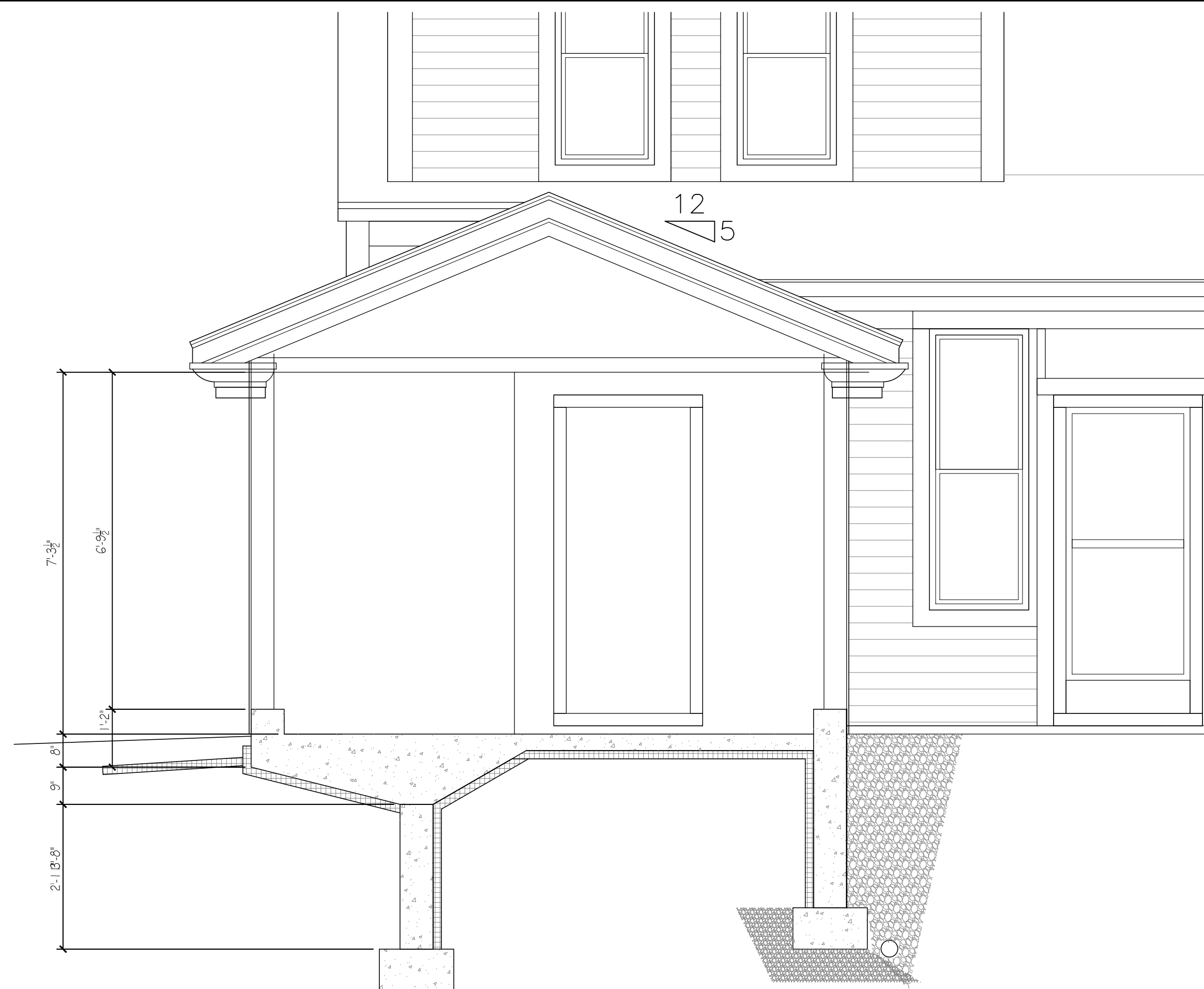
SECTION @ SLAB CANTILEVER SCALE: 1/2"=1'-0"
