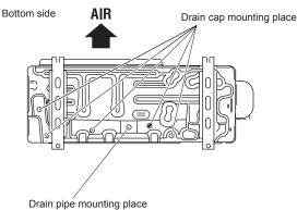
Since the drain water flows out of the outdoor unit during heating operation, install the drain pipe and connect it to a commercial 16 mm hose. (Reverse cycle model only) When installing the drain pipe, plug all the holes other than the drain pipe mounting hole in the bottom of the outdoor unit with putty so there is no water leakage. (Reverse cycle model only)
