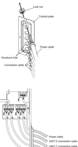
UNIT C connection cable UNIT C connection cable UNIT A connection cable
