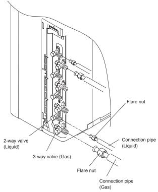
When the flare nut is tightened properly by your hand, use a torque wrench to finally tighten it
