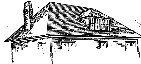
Fig. 242. Hip Roof with Ridge
